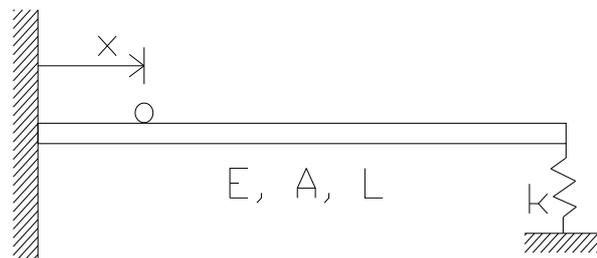
Figure 1: Beam with a moving mass and elastic end constraint
