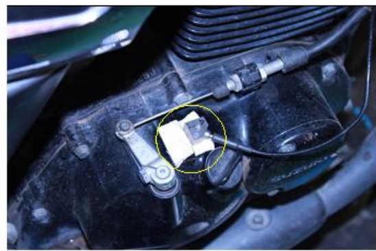
Fig.7. Engine Casing vibration measurement by Tri-axial accelerometer
