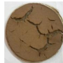
(b) Cracking pattern of bentonite with 0.4M CH 3 COOH (air dry)
