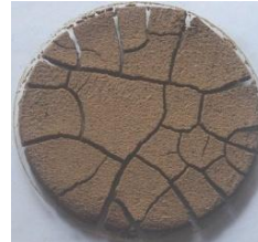
(b) Cracking pattern of bentonite with 0.4N NaOH (air dry)
