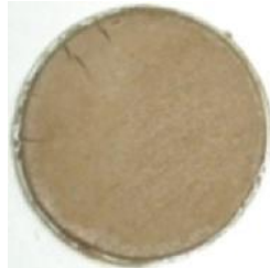
(a) Cracking pattern of bentonite with 0.1N NaOH (air dry)
