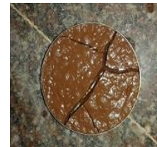
(b) Cracking pattern of bentonite with 0.4M NH 4 Cl (air dry)
