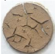
(a)Cracking pattern of bentonite with 0.1M CH 3 COOH (air dry)
