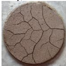
(a)Cracking pattern of bentonite with 0.1M NH 4 Cl (air dry)
