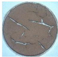
(a)Cracking pattern of bentonite with 0.1M NaCl (air dry)
