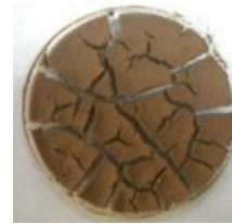
(b) Cracking pattern of bentonite with 0.4M NaCl (air dry)
