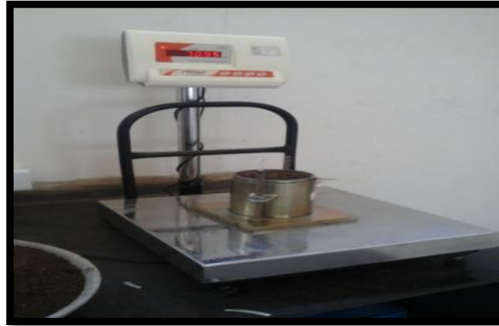
Figure 3: Modified proctor test
