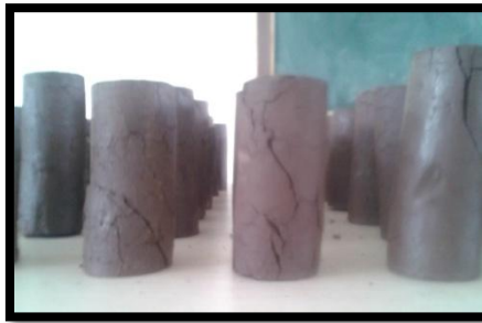
Figure 4: Failed samples when subjected to loading
