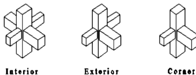
Fig 1: Types of beam column joints (source: ACI 352R-02)
