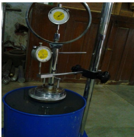
Fig.8 Swelling testing machine
