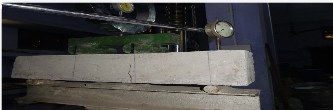
Fig. 7 Flexural strength surface of recycled aggregate concrete
