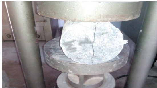
Fig. 5 Split tensile failure surfaces of Recycled aggregate concrete
