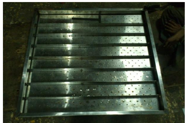
(b) Actual photo of adsorbent bed
