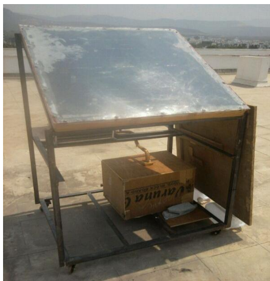
Fig. 10 Actual system of ice-maker
