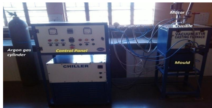
Fig 2.1- Set up of vacuum stir casting furnace
