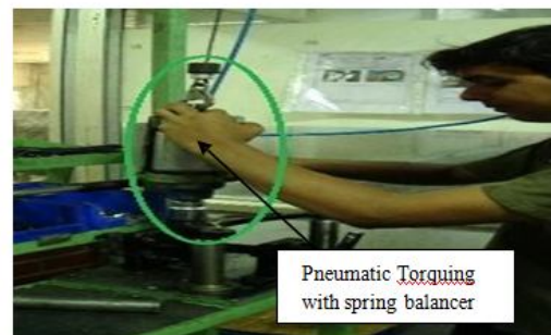
Fig 8. Pneumatic torquing After implementation
