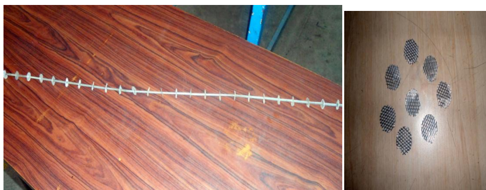
Fig.2 Mesh inserts manufacturing
