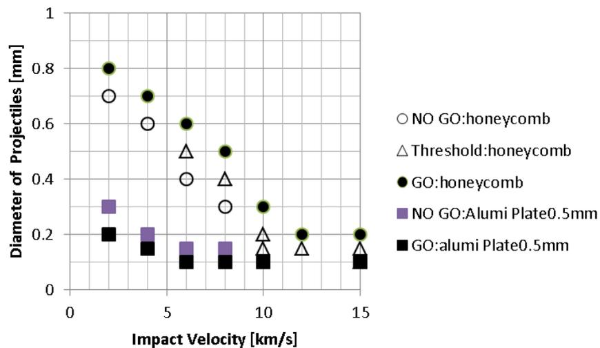
Fig. 7 Numerical simulation results for various projectile diameter and impact velocity
