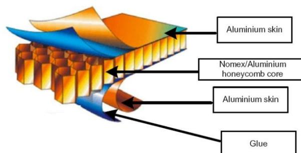
Fig. 1 Honeycomb Sandwich Panel
