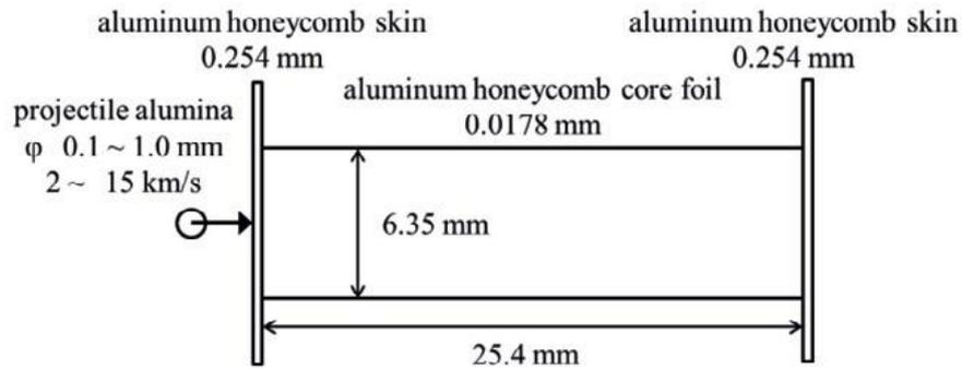
Fig. 5 Two dimensional axial symmetry analytical model
