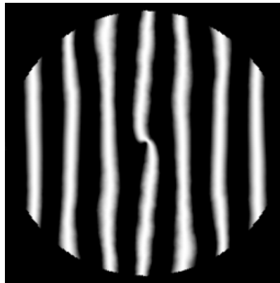
Fig. 4: Representation of interference fringe pattern with a turbulent phasescreen of D/r_0 = 0.2 .
