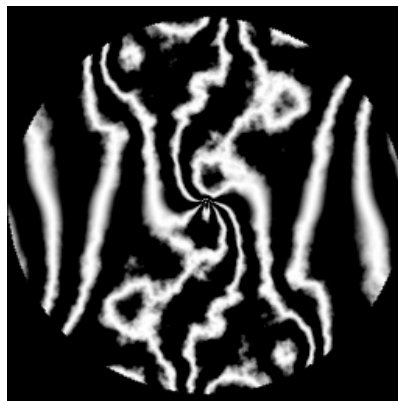
Fig.5: Representation of interference fringe pattern with a turbulent phasescreen of D/r_0 = 2.5 .
