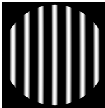
Fig. 3: Representation of straight interference fringe pattern in the absence of turbulence with D/r_0 = 0 .
