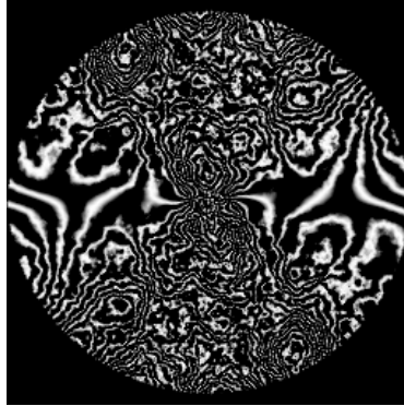
Fig. 6: Representation of interference fringe pattern with a turbulent phasescreen of D/r_0 = 25 .
