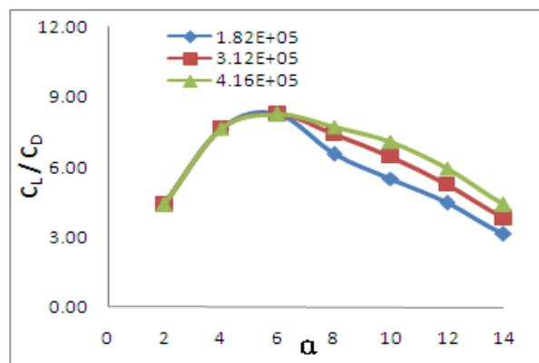
**Fig 9-**  $C_L / C_D$  with angle of attack
