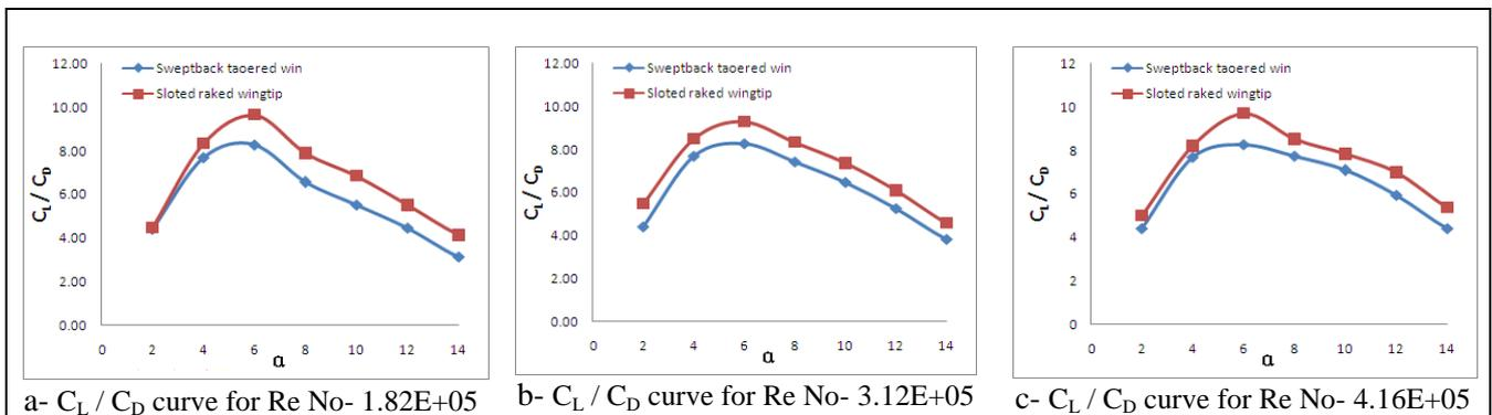
Fig 13- Variation of aerodynamic efficiency ( $C_L / C_D$ )
