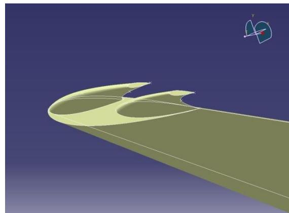
**Fig 3-** Single Slotted Raked Wingtip (second configuration).
