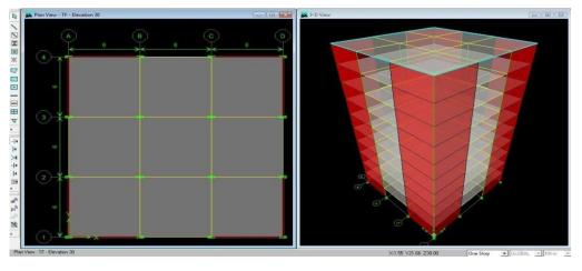
Plan View 3-D View Fig. 4.4 showing G + 9 Storey Building with Shear wall
