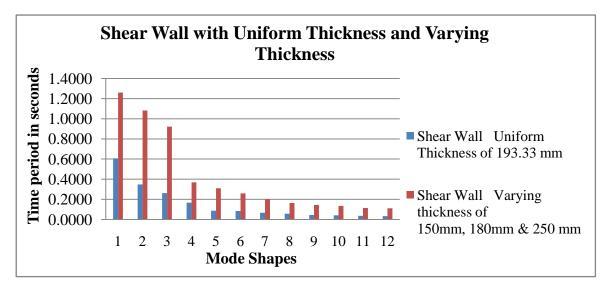
Fig.4.13 Shear wall with Uniform Thickness and Varying Thickness
