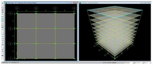
Plan View 3-D View Fig. 4.5 showing G + 9 Storey Building without Shear Wall
