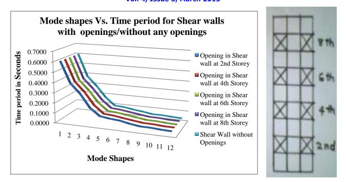
Fig. 4.15 3D Line Graph showing Mode Shapes Vs. Time period for Shear Wall with openings (2, 4, 6, 8 Stories) / without openings
