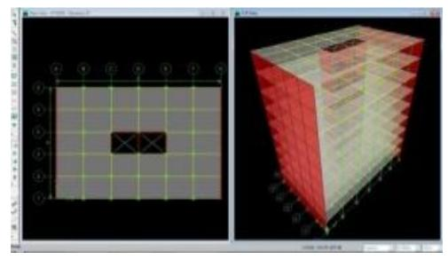
Plan View3-D ViewFig. 4.12 showing G + 9 Storey Building with Shear Wall & Lift core wall
