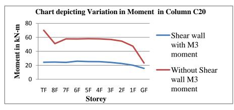
Fig.4.11 Moment distribution for different Storey's
