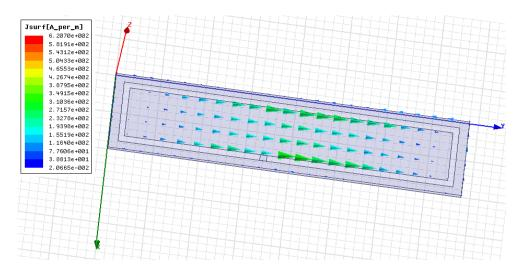
Fig 7: Surface current distribution of E-field
