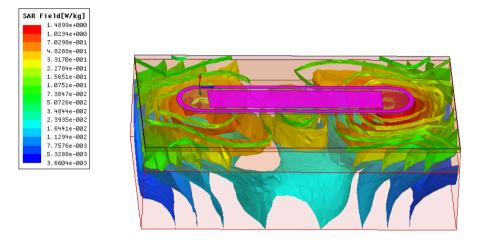
Fig 3: Specific Absorption Rate on a body phantom
