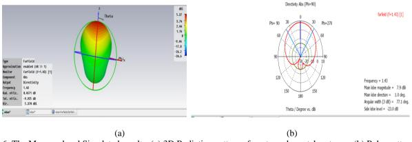
Fig 6: The Measured and Simulated results (a) 3D Radiation pattern of rectangular patch antenna. (b) Polar pattern of rectangular patch antenna.
