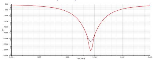
Fig 5: Magnitude of S11 for Microstrip antenna with polyimide
