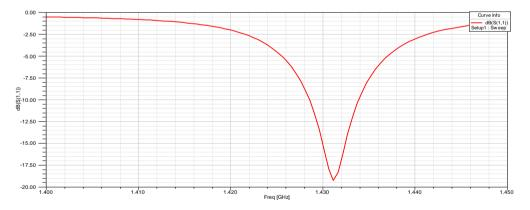
Fig 4: Magnitude of S11 Vs Frequency for Square Patch Antenna.
