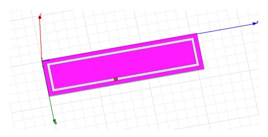
Fig. 1. Original design of Microstrip patch antenna.
