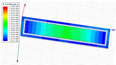
Fig 8: Surface current distribution of H-field
