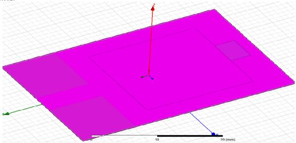
Fig 2: Microstrip antenna with polyimide substrate
