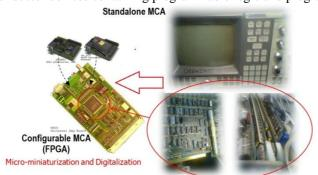
Fig. 1: Miniaturization and Digitization of MCA Canberra series 35 plus electronics
