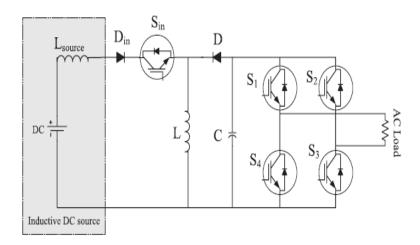
Fig. 3 Converter topology connected to DC nature of the source
