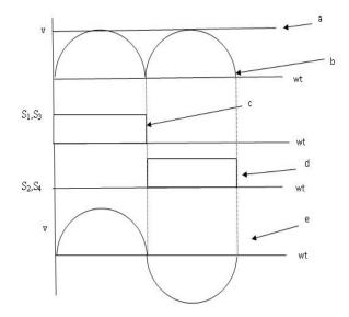
$\begin{array}{l} \mbox{Fig. 4 The operational characteristics of converter topology: a) DC input voltage, b) Output of boost converter, c) Switching pulses to S_1, S_3, \\ \mbox{ d) Switching pulses to } S_2, S_4, e) Output voltage of inverter \\ \end{array}$
