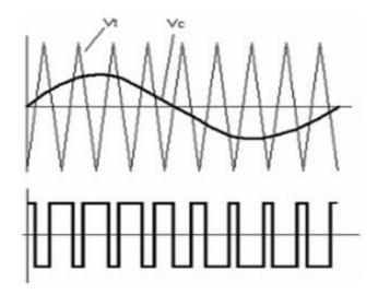
Fig. 5 Generation of pulses for switches
