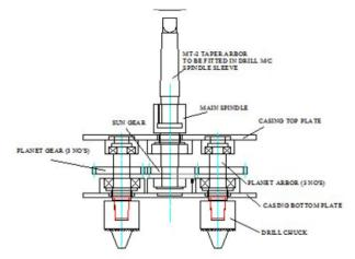
Fig 2.1 Principle of Twin Spindle Drilling
