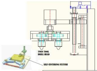
Fig 5.1 construction of Twin drill head machine
