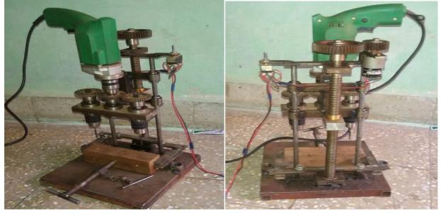
Fig 7.1 assembly of Twin drill head with depth control machine
