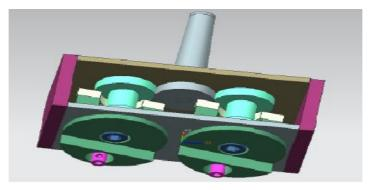
Fig 2.2 Principle of Twin Spindle Drilling in 2D
