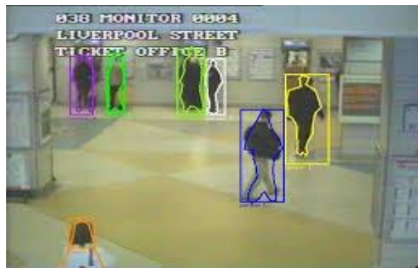
Fig.7 Object tracking using region based technique
