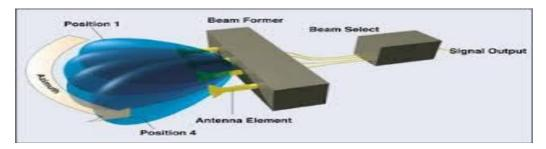
Based on the type used there are two types of smart antenna \*Switched multibeam antenna(figure a) \*Adaptive array(figure b)
