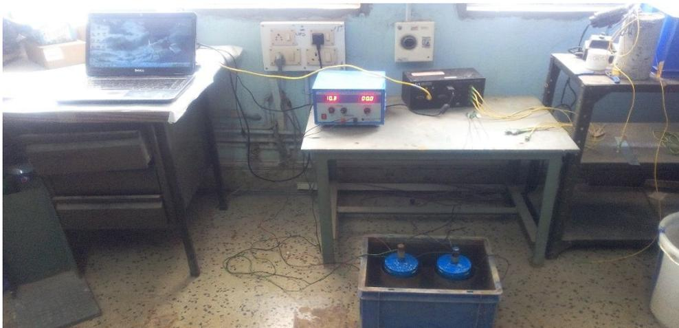
Fig 9: Accelerated corrosion of specimen 1 & 2 after Epoxy Coating
