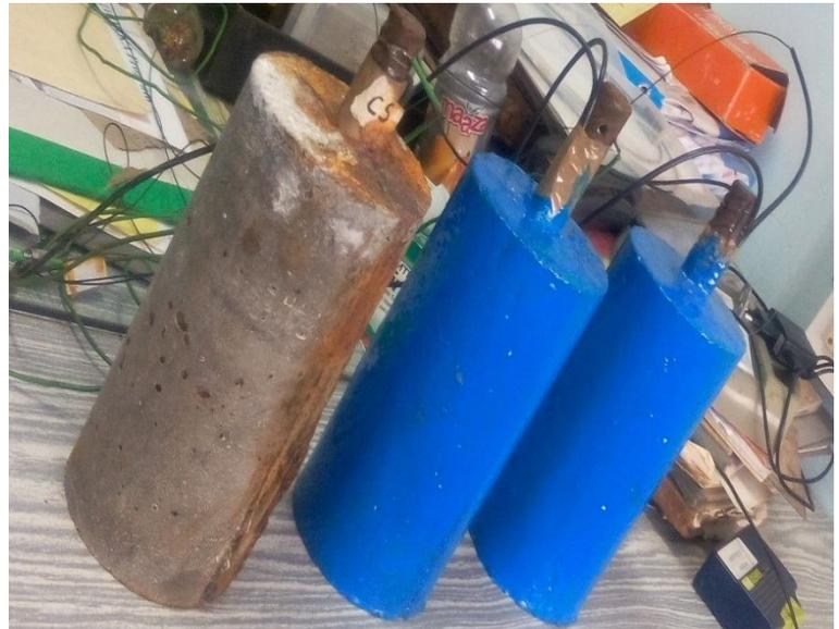
Fig: 8 Specimens Treated with Epoxy Coating and Control Specimen
