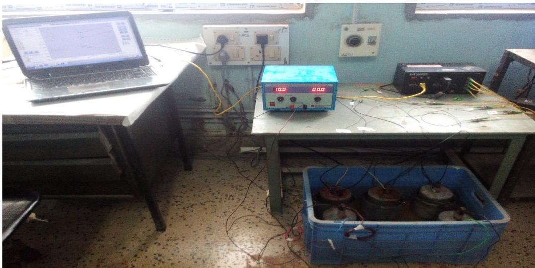
Fig. 5 Accelerated corrosion test set up
