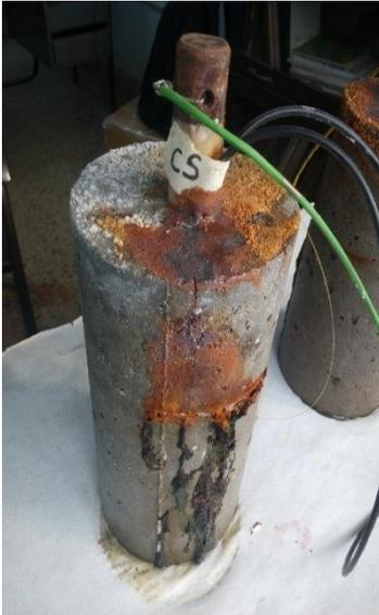
Fig. 7 Control Specimen after Cracking
