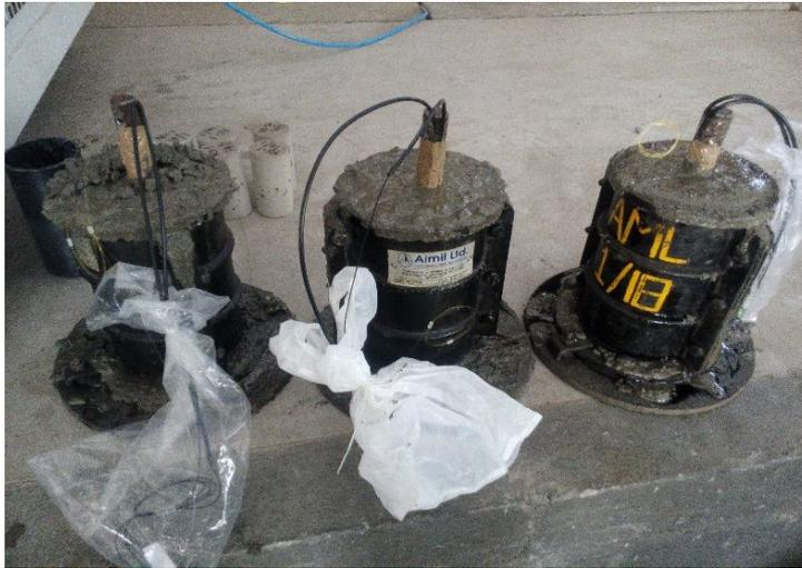
Fig.4 Embedding of FBG instrumented rebar
