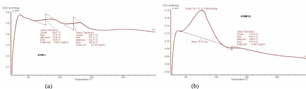
Fig. 2 Thermal properties of (a)PBAZBT (b) PBAZBT blend
