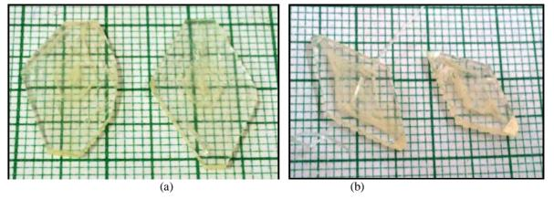
Fig. 1. Bulk Crystal grown by (a) Solvent evaporation method (b) Slow cooling method
