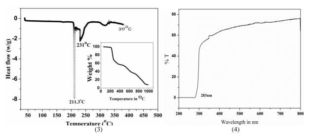
Fig. 3. DSC curve for BTCC and the inset shows the TGA curve for the complex Fig 4. UV- Visible spectrum of BTCC
