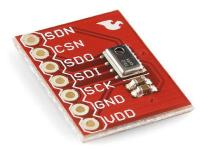
to a system which uses an inter integrated circuits for communication . It is a monolithic temperature sensor that generates a modulated serial digital output (PWM) which varies in direct proportion to the temperature of the devices. T. It offers a high temperature accuracy of  $\pm 1^{\circ}$ C from -55 to 150°C with excellent transducer linearity.
