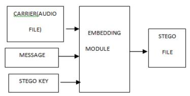
• The basic model of Audio steganography consists of Carrier (Audio file), Message and Password.
