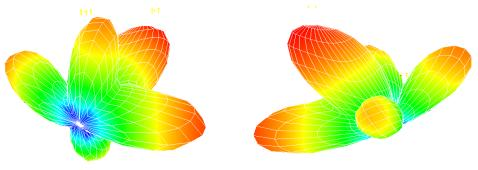
Fig. 2 (c) Gain Pattern of Circular Patch
