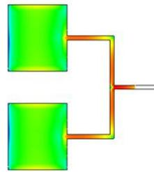
Fig. 1(d) Current Density of 2x1 Array
