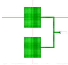
Fig. 1(c) Meshed Patch of 2X1 Array
