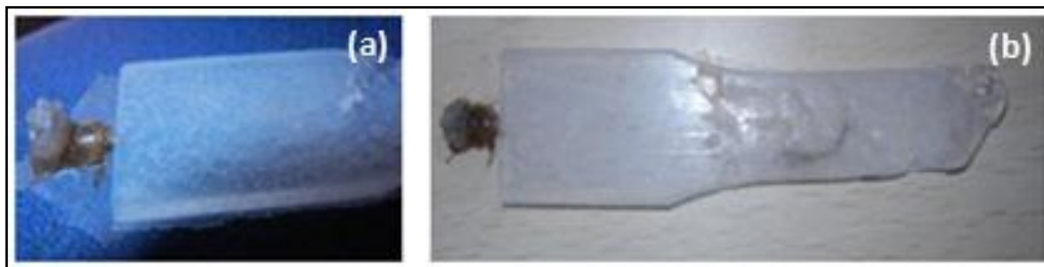
Fig. 9: (a) Fiber clogging, (b) Short shot
