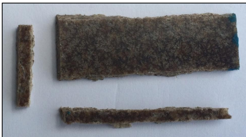
Fig. 4: Cut sample for Micro-Tomography
