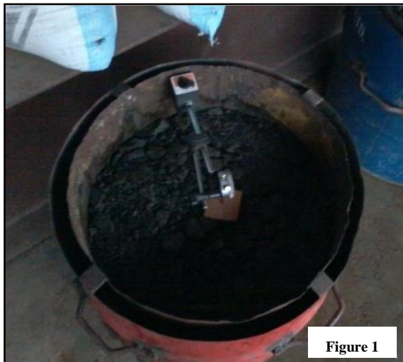
Fig: 1 Heave measurement setup in model pavement system tanks Fig: 2 Sectional 3d view of model pavement system laid in laboratory
