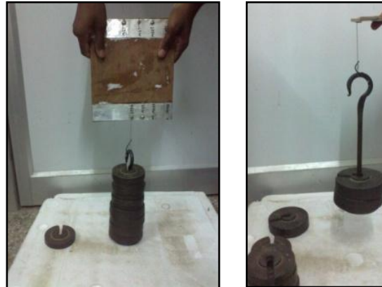
Fig. 1 Photographs of suspended weights along and perpendicular direction of the soldered point are shown from left to right [5].
