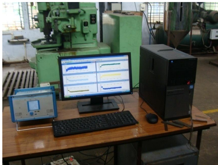
Figure: 3 Experimental Set up for measuring the cutting force
