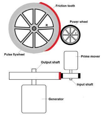
Fig: 2 Construction of pulse mechanism for power generation.
