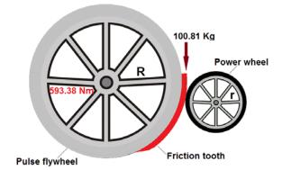
Fig. 5: relation of torque between power wheel and pulse wheel
