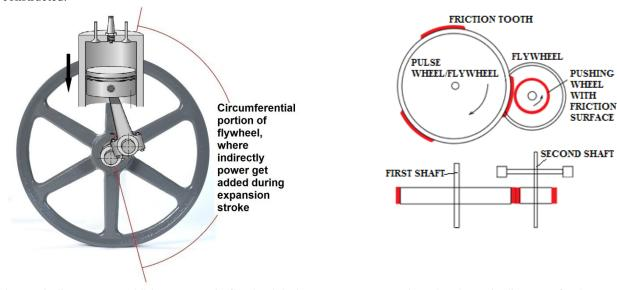
Fig. 1(a)indirect power addition process in flywheel during expansion stroke
