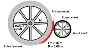
Fig.4: considered radial ratio for pulse flywheel and power wheel.
