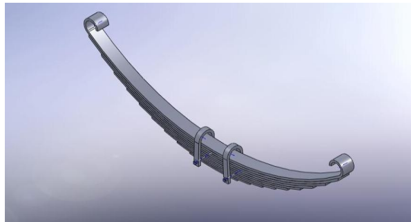
Figure.1 3D view of Existing Leaf spring
