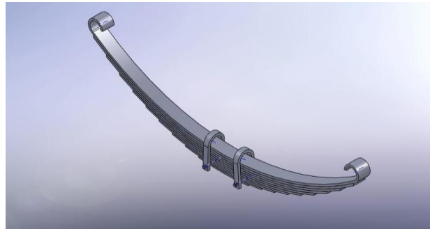
Figure.2. 3D view of modified Leaf spring
