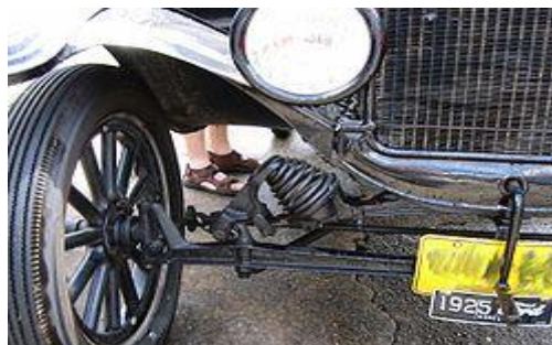
The front suspension components of a Ford Model T.
