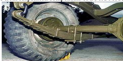
The rear suspension on a truck: a leaf spring.
