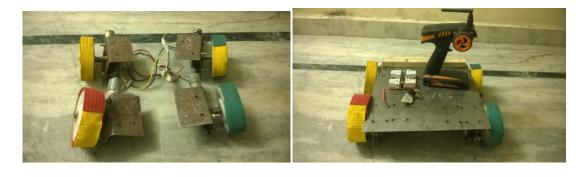
(a) (b) Figure 6 :- (a) assembling process of wheels with clamp and wires connection (b) A set of assembled wireless robot
