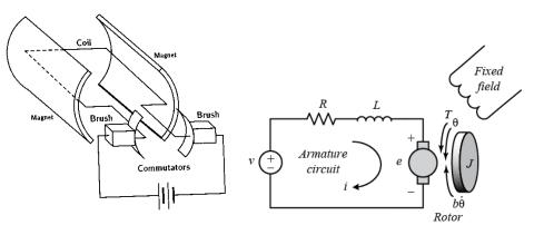
Figure 1 :- Circuit diagram of a DC motor
