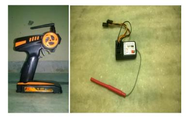
(a) (b) Figure 2 :- (a) Transmitter ), (b) receiver
