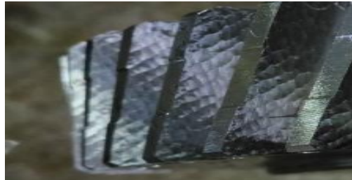
Figure 4: No Patch marks and Varied Crossed Feed marks evident after hobbing operation
