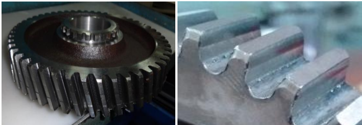
Figure 1: Gear having root step problem
