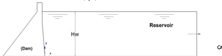
Fig.1 Rigid dam-infinite reservoir system
