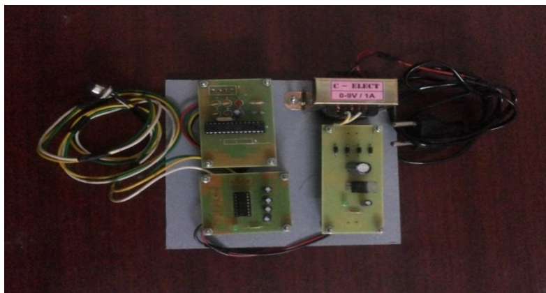
Figure 4: Experimental setup of Digital pen Receiver
