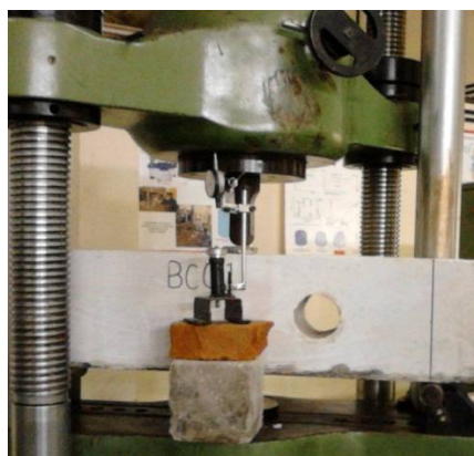
Fig.2. Flexural test setup
