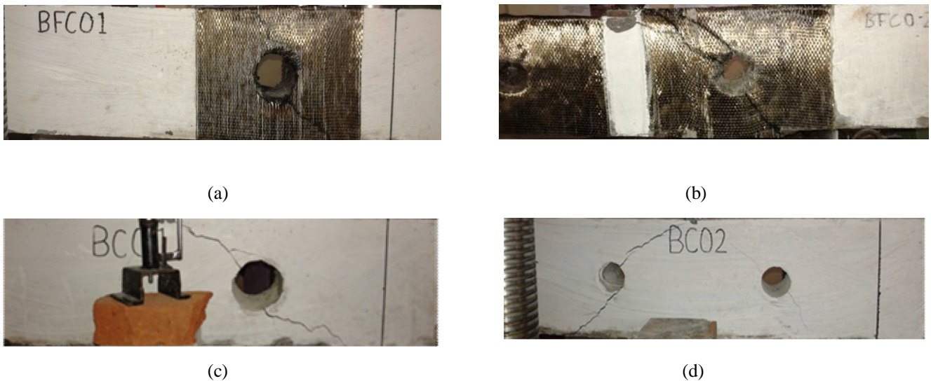
Fig.3.crack pattern(a)strengthened beam with one cicular opening(b) strengthened beam with two circular opening (c)unstrengthened beam with one cicular opening(d) unstrengthened beam with two circular opening.
