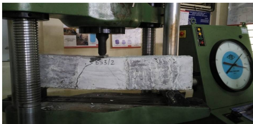
Fig. 4. Test set up for beam specimen
