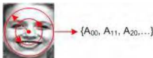
Fig.4 Example of ZM for feature extraction with different orders and repetition
