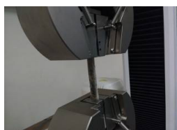
Figure 6: Tensile testing in UTM
