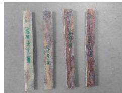
Figure 9. Flexural Testing Specimens
