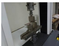
Figure 8. Flexural Testing in UTM
