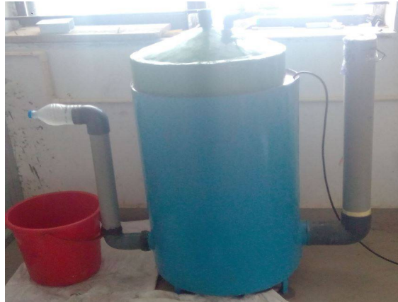
Fig.2 Photograph of metal made biogas plant
