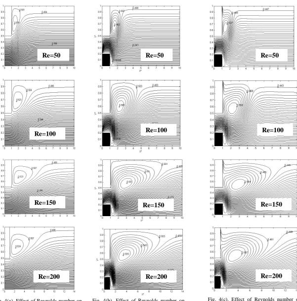
Fig. 4(a). Effect of Reynolds number on streamline contour for AR=2 and CR=0%
