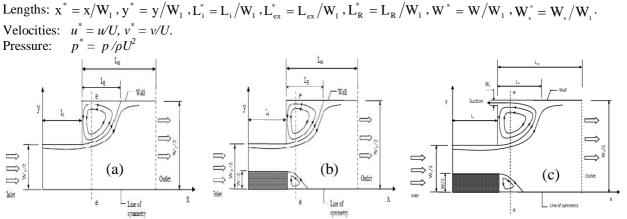
Fig. 1. Schematic diagram of the computational domain (a) plain sudden expansion (b) sudden expansion with central restriction only (c) sudden expansion with central restriction and suction
