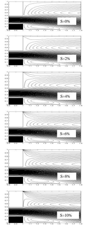
Fig. 2(b) Effect of suction on streamline contour for AR=2, Re=100 and CR=40% (enlarged view of central region)
