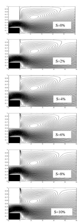
Fig. 2(a) Effect of suction on streamline contour for AR=2, Re=100 and CR=40\%
