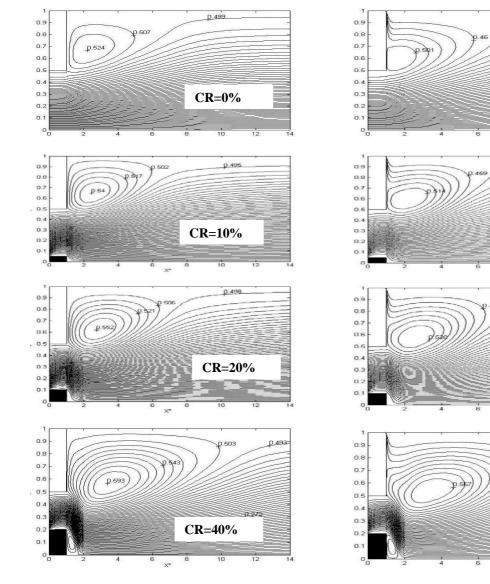
Fig. 3(a). Effect of central restriction on streamline contour for AR=2 and Re=200  $\,$
