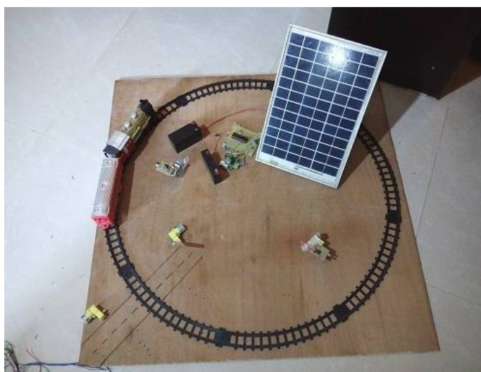
Fig 8. Model hardware implimentation Of automatic railway gate controller.
