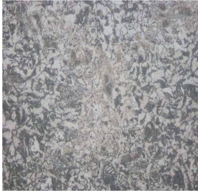
Fig: microstructure of oil quenched specimen at 500X
