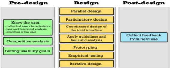
Figure 2. The stages of the usability engineering lifecycle model
